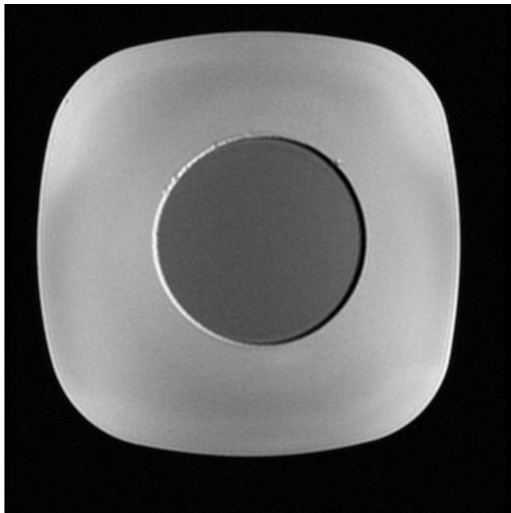
The images above are of a phantom made from tap water (outer circle) and olive oil (inner circle) with a T2 weighted FSE. Bandwidth is increased from 10 kHz up to 63 kHz. Notice with low bandwidths the SNR is high, but the chemical shift artifact is significant
